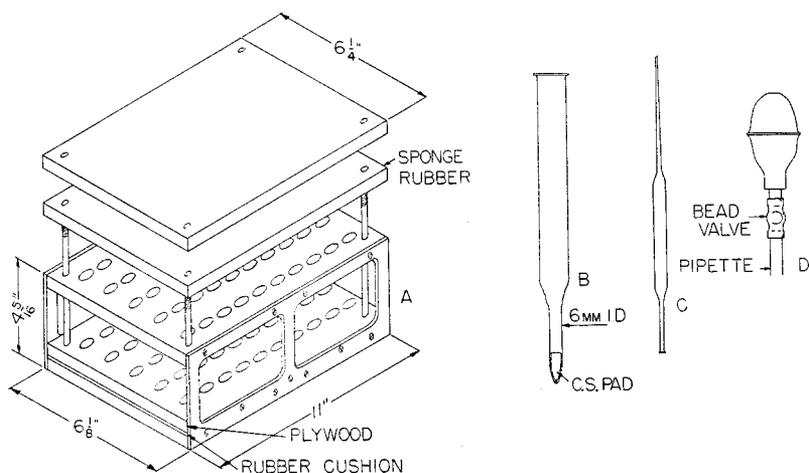
FIG. 2. A, special holder for shaking glass-stoppered test-tubes (the bottom, center, and top plates are made of  $\frac{1}{8}$  inch aluminum plate; the sides are of  $\frac{3}{16}$  inch aluminum plate); B, CS tube with 100 mg. CS pad; C, glass weight which rests on CS pad to keep it firmly packed; D, pipetting bulb arrangement.
