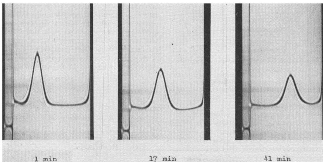
FIG. 2. Sedimentation velocity pattern of 2-keto-3-deoxy-6-phosphogluconic aldolase after 1, 17, and 41 minutes at 59,780 r.p.m. The enzyme (10 mg per ml) was dissolved in 0.05 M phosphate, pH 6.0, and 0.15 M NaCl. Direction of sedimentation is to the right.
