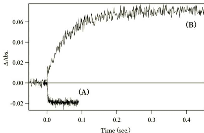
FIG. 1. Transient absorbance changes at 420 nm obtained after a 355-nm laser excitation of Pdx<sup>ox</sup> (A) and ferric P450cam (B) at 293 K. The sample solution contains 10  $\mu\text{M}$  protein in 50 mM KP<sub>i</sub>, 1 mM *d*-camphor, 15  $\mu\text{M}$  acridine, 500  $\mu\text{M}$  MV, 25 mM EDTA, pH 6.7
