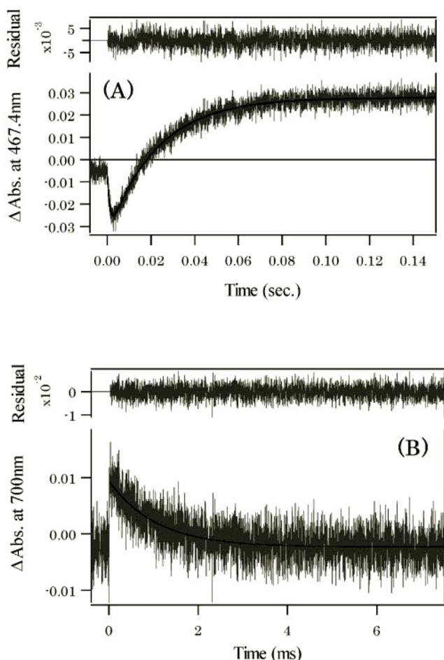
FIG. 3. Transient absorbance change at 467.4 nm (A) and 700 nm (B) obtained after a 355-nm laser pulse. The residuals of the double-exponential (A) or the single-exponential (B) fitting are shown at the top of the figure. Conditions; 10  $\mu\text{M}$  Pdx<sup>ox</sup>, 20  $\mu\text{M}$  P450cam in 50 mM KP<sub>i</sub>, 1 mM *d*-camphor, 15  $\mu\text{M}$  acridine, 500  $\mu\text{M}$  MV, 25 mM EDTA, pH 6.7.
