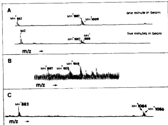
FIG. 4. Partial positive ion FAB-MS spectra of the purified pineal OT1 (A), OT2 (B), and VP1 (C). The protonated molecular ions (MH<sup>+</sup>) for each peptide are indicated by arrows. \*, sodiated ion (MNa<sup>+</sup>) of formylated oxytocin; \*\*, sodiated ion (MNa<sup>+</sup>) of acetylated oxytocin.
