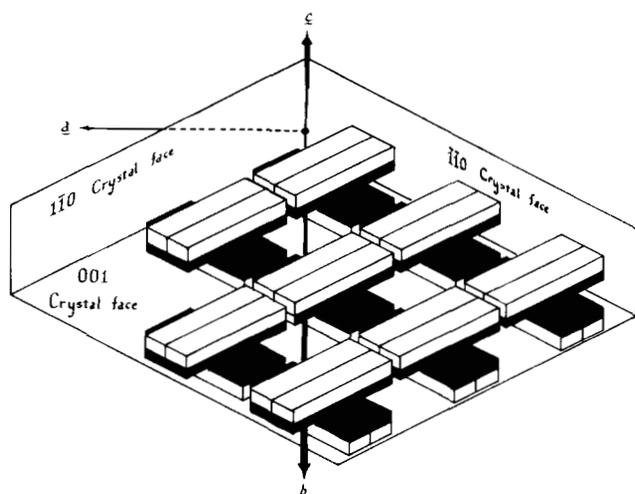
FIG. 5. Packing of melittin chains in the form II crystals. Each tetramer is schematically represented by four crossed blocks. The shaded side represents the side of the melittin chain which is hydrophobic for residues 1–20. The faces of the form II crystals are related to the packing of the tetramers. One face is perpendicular to the  $c$  axis; it is the surface of a sheet of tetramers. The other two faces are parallel to the  $c$  axis and to two of the chains in each tetramer.
